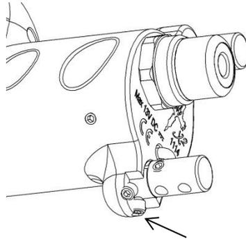
Remove the **Clip cord binding post positive (+) ⑩** and the sleeve. Replace if necessary.
