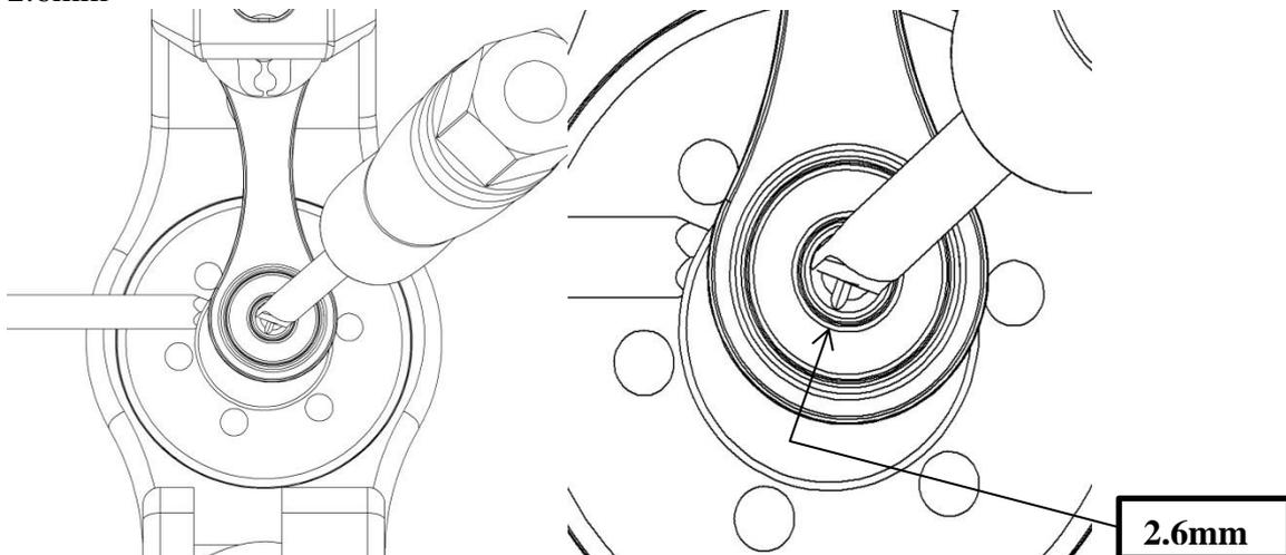
When the stroke has been selected and the pin is in the correct position tighten the screw just a bit. Twist the screw driver and the Eccentric pin back and forth to make sure that the screw seats on a flat part of the Eccentric pin. There is one flat part for each stroke position as you can see on the cut through section of the Eccenter below. Do not over tighten the screw.
