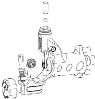
4. Refit only the **Adjustment screw** ⑱ a few turns and push the **Piston assembly** ④ down to the bottom position by pushing on the top of the adjustment screw.
