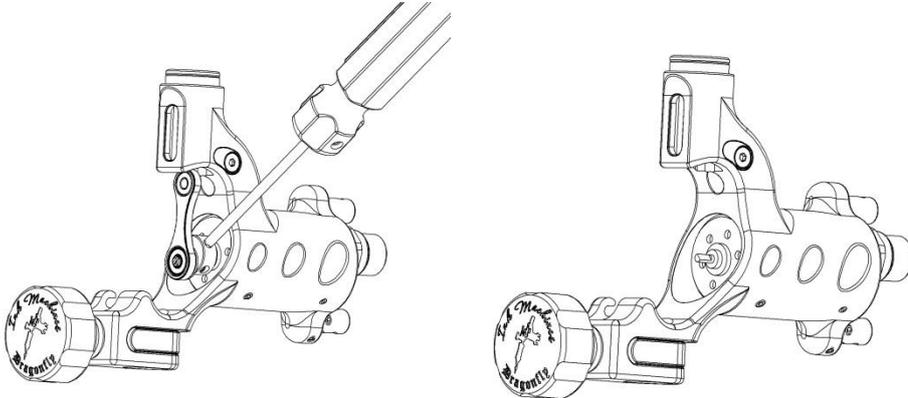
9. Loosen the **Contact screw cord positive (+)** ⑰ and pull out the cord end. Loosen the **Motor fixing screws** ⑭ and **Contact screw motor negative (-)** ⑯ and pull / push out the **Motor assembly** ④② ③.
