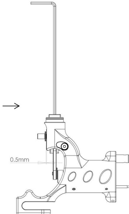
9. Insert the **Inner piston spring** ⑲, screw in the **Adjustment screw** ⑳ all the way down. Align and push the **Cap** ③ ⑧ in to place. Move the **Cap** ③ ⑧ in a circular motion while pushing to make it snap in to place.
