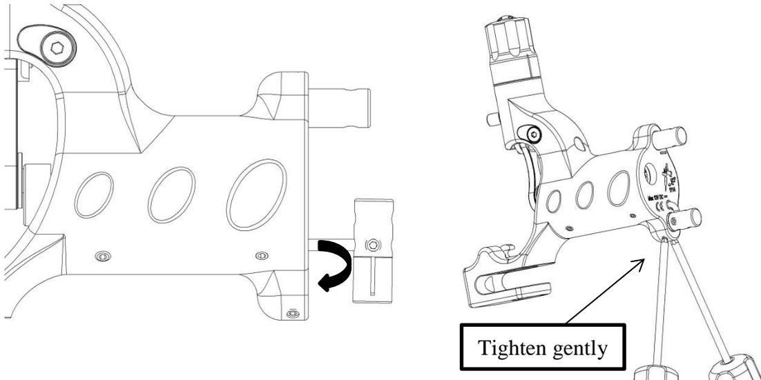
11. Install the **RCA contact ⑫** and **RCA nut ⑬** by turning the RCA contact until the tip touches the contact plate of the motor gently. Tighten the RCA nut gently.
