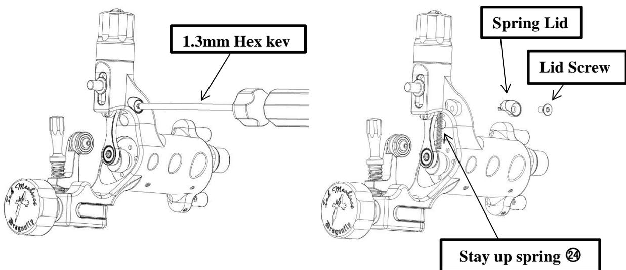
To take advantage of the give function when using cartridges the Inner piston spring should be replaced. If the give function is not required just adjust the give to the bottom position (hardest setting).
