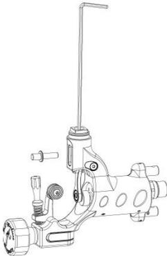
3. Push out the **Inner piston** ㉑ and pull out the **Noise damper O-ring** ㉒ from the bottom of the **Piston** ㉑.
