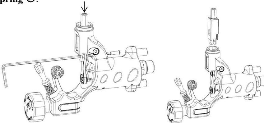
7. Remove the **Needle bar retainer assembly 44** by unscrewing the **Retainer fix. Screw 48** and pulling it out.
