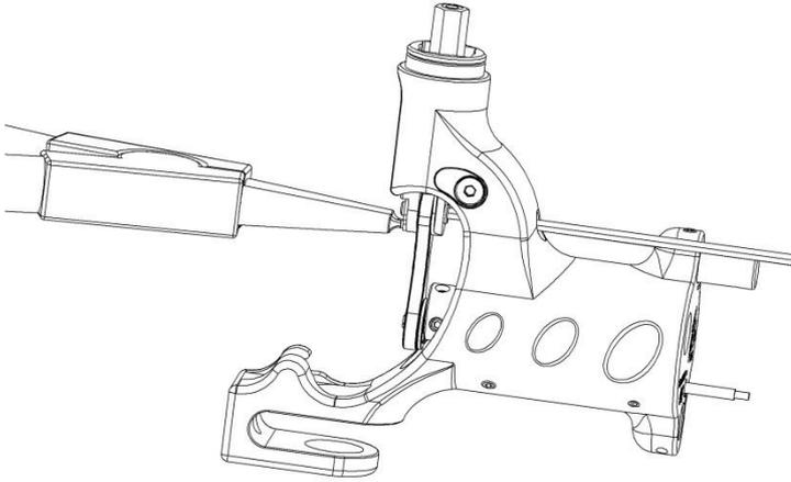
7. Install the **Noise damper O-ring** ㉗, push it to the bottom of the hole in the **Piston** ㉑ and make sure it lies firmly in the bottom. Align the **Inner piston** ㉘ with the **piston screw** ㉙ pointing up and the **Needle bar pin** ㉚ hole pointing in the direction of the groove in the **Frame** ①. Push it down to the **Noise damper O-ring** ㉗.
