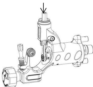
5. While holding the **Piston assembly 40** in the bottom position, remove the **Circlip 25** from the **connecting pin 23** with a **Circlip pliers 55**. Don't open the circlip more than it exactly needs to clear the connecting pin or it will overstretch and become useless. Use a **Circlip pliers 55** with an adjustable stop screw that prevents the circlip from opening too much.
