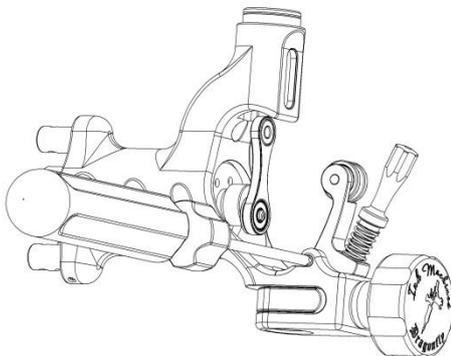
8. Loosen the Allen screw in the **Eccenter** ⑧ that holds the motor shaft. Pull out the **Eccenter assembly** ④① ⑧ from the motor shaft.
