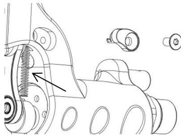
The hexagon of the **Adjustment screw ⑧** is damaged and pivots inside without the cap following.
