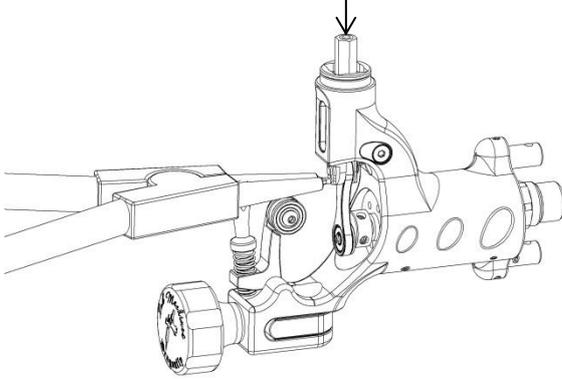
6. Use a 1,5mm pin or the far end of an **Allen key 54** to push out the **Connecting pin 23** out and through the hole in the **Frame 1**. Pull out the **Piston 21** and the **Stay up spring 24**.
