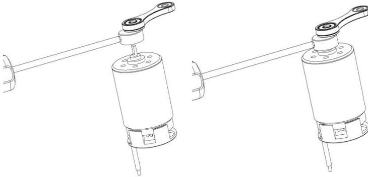
2. Insert the **Motor assembly** ④⑧ into the **Frame** ① while aligning the motor cord to the corresponding hole at the back of the **Frame** ①.
