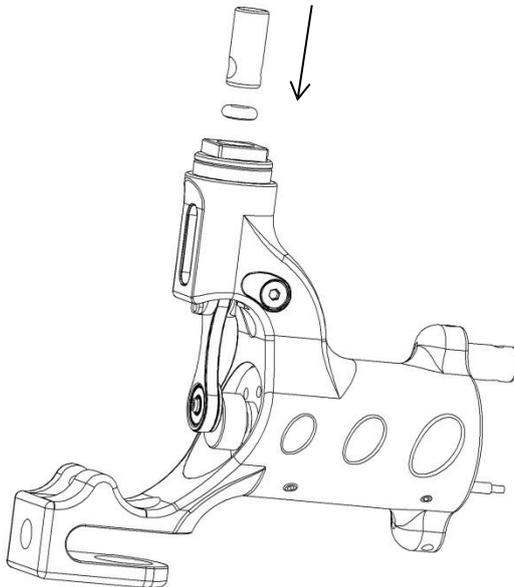
8. Insert the **Needle bar pin** ⑥ through the groove of the **Frame** ① and through the hole of the **Inner piston** ⑳. The distance between the sleeve of the needle bar pin and the **Frame** ① should be approx 0,5mm. Tighten the needle bar pin with the **Allen key** ⑤4 from the top.
