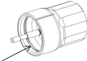
The needle bar retainer O-ring is not round.
