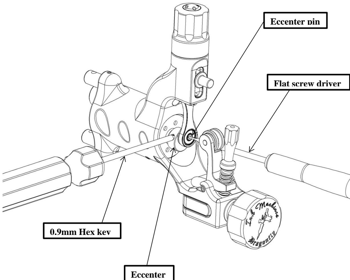
Loosen the screw from the side of the Eccenter ⑧ min 2 turns. Twist the Eccenter pin 90 or 180 degrees to the desired location and corresponding stroke length.
