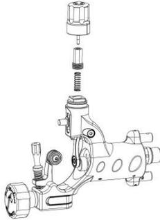
2. Use the matching **Allen key** ④ to loosen the **Piston screw** ⑳ in the **Inner piston** ㉑. Take out the **Needle bar pin** ⑥.
