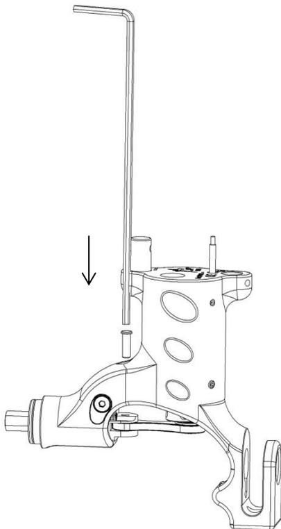
6. While holding the **Piston** ⑳ at its bottom location keep pressure on the head of the **Connecting pin** ㉓ with the far end of an **Allen key** ㉔. Install the **Circlip** ㉕ using a **Circlip pliers** ㉖.
