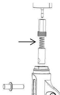
Too much play between the **Piston** ㉑ and the **Inner piston** ⑳. (worn out ).
