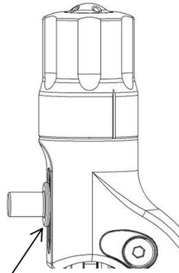
**Needle bar retainer bearings ㉓** worn or clogged.
