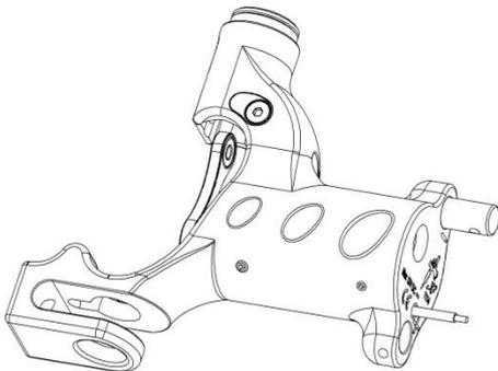
3. Lubricate and insert the **Piston** ②① with the **Stay up spring** ②④ and the **Adjustment screw** ⑩ into the **Frame** ①. Make sure the stay up spring aligns with the **Lid** ⑨⑤.
