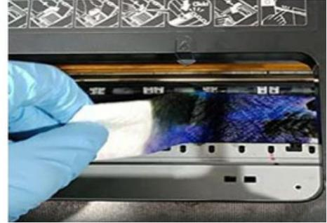
7. Allow the solution to soak for approximately 1 hour to dissolve the blockage. Repeat the cleaning process as needed for each colour.
