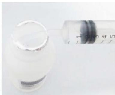
5. Draw 2-3 ml of cleaning solution into the included injection syringe.
