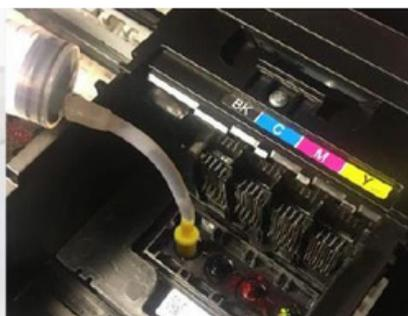
6. Using the provided attachment, carefully dispense the solution through the corresponding nozzle. Repeat for all colours.
