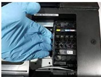
2. Select "Replace Ink Cartridge" and wait for the carriage to move into position. Unplug the printer and push the carriage to the right side.
